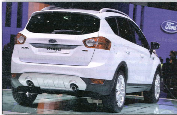
The thermal expansion of parts made with LyondellBasell's HiFax TRC 280X mineral-filled PP is said to be low enough to allow the compound's use for the Ford Kuga's tailgate outer panel (above) and roof spoiler (opposite page). LyondellBasell.
